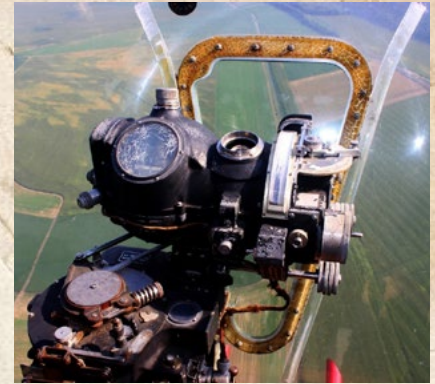
The view from the front and the Norden Bombsight
